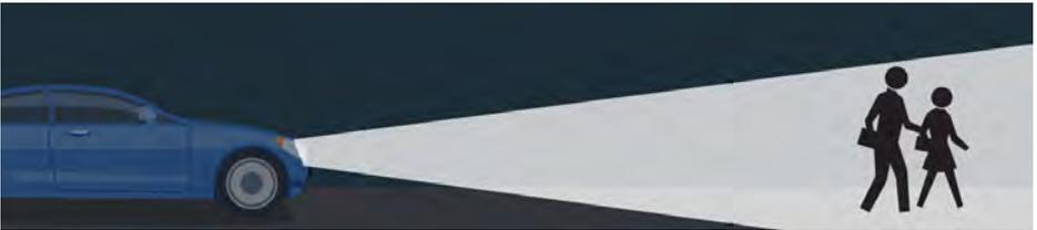
High beam headlights can reveal objects up to a distance of at least 450 feet and are most effective for speeds faster than 25 MPH.
